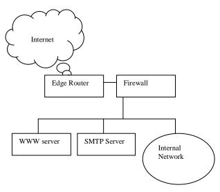
Fig 4. Common IPv4 network
